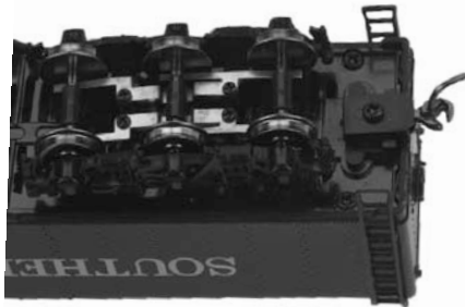
Insert the coupler (as shown) and screw into place
