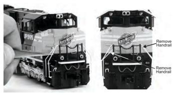
Then remove the handrails on the left and right side front of the engine. You can either remove the stanchions from the body or pop the handrail off the stanchions. Use tweezers or needle-nose pliers to carefully perform this. To prevent damaging the paint wrap the pliers or tweezer tips in masking tape. Take care not to deform the handrail or break the handrail stanchions.
