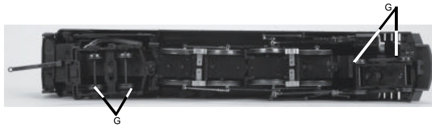
Figure 11: Greasing the leading and trailing truck pivot points.
