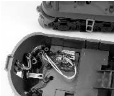
Figure 23: Wire harnesses connect lights inside the locomotive body.
