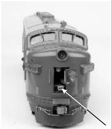
Figure 28: Battery Recharging Port
