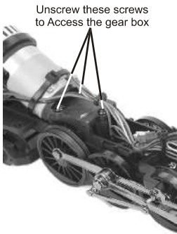
Figure 7. Motor Gearing Grease Plate Screws
