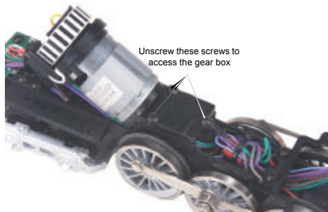
Figure 7: Motor Gearing Grease Plate Screws
