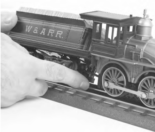
Figure: Attaching the Plastic Drawbar Holder
