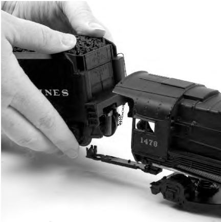
Figure: Connecting Locomotive to Tender
