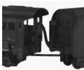
Figure 1: Plugging in the tender harness
