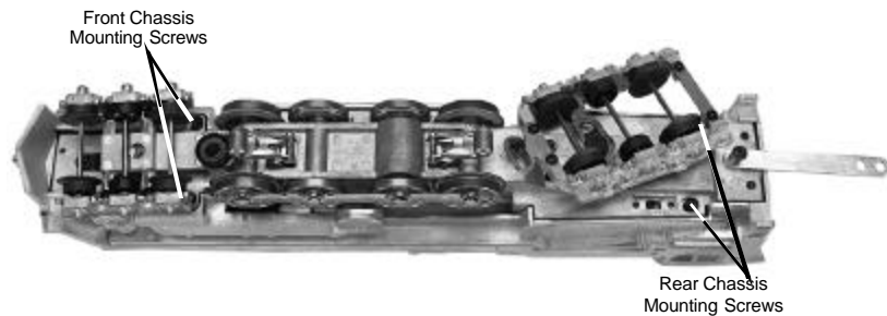
Figure 10: Removing The Boiler From The Chassis
