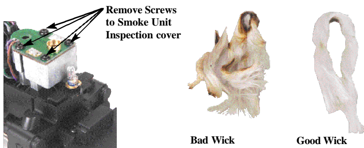
Figure 8 - Inspecting the Smoke Unit
