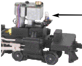
Figure 9 - Replacing Headlight Bulb
