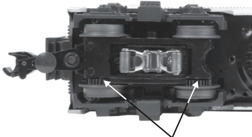
*Greasing The Idler Gears*
