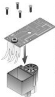
Figure 21: Opening the smoke unit for wick replacement.
