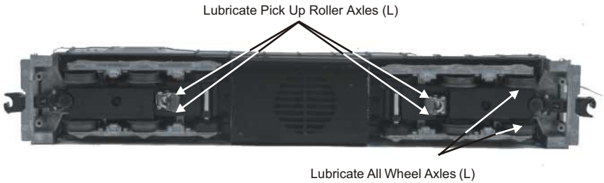
Figure 1. Lubrication Points on the Locomotive
