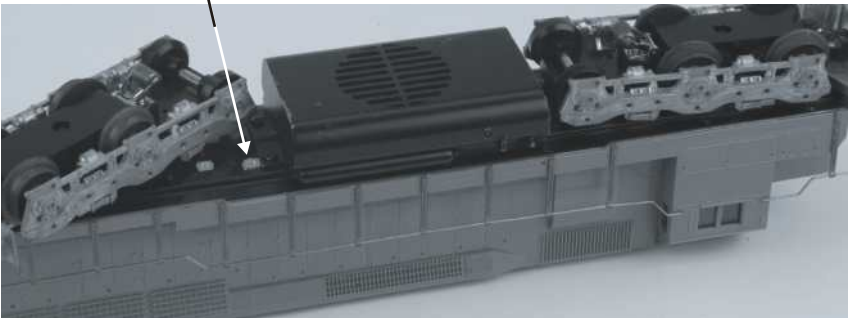
Figure 4. Manual Volume Adjustment Knob
