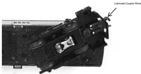
Figure 3: Lubricating The ProtoCouplers
