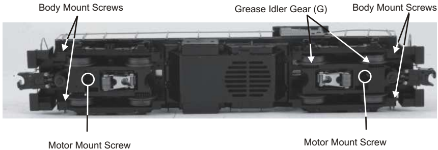
Figure 5. Body Removal Screw Locations
