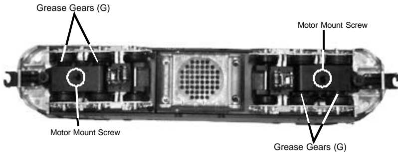
Figure 7: Greasing the Power Trucks
