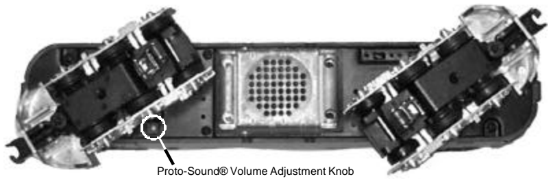
Figure 4: Adjusting The ProtoSound Volume and selecting the ProtoCoupler™
