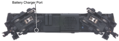
Figure 6: Battery Charger Port
