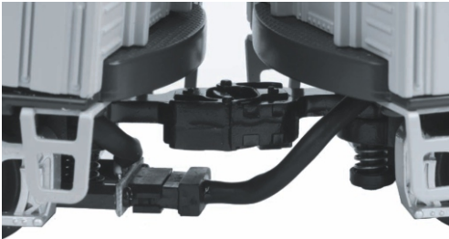
Correct way to Connect wire harness plug into the receptacle
