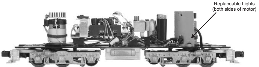
Figure 8b: Replacing the Lights in your Engine
