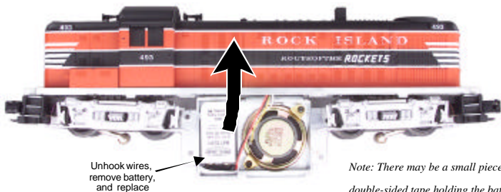
Figure 6. Removing and Replacing the Battery
