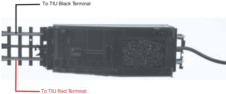
Figure 5: Proper 2-Rail polarity wiring and locomotive orientation
