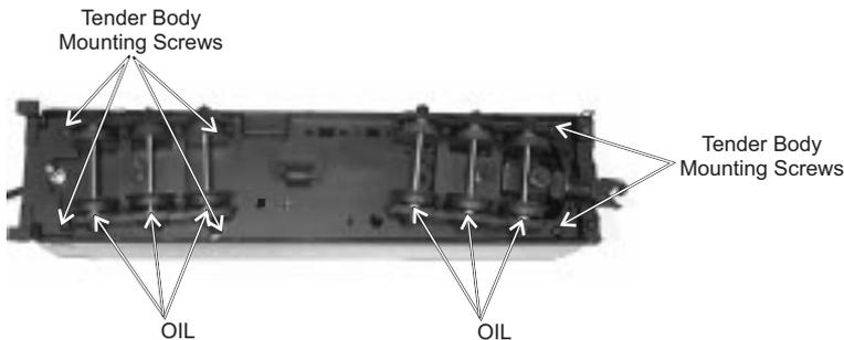
Figure 9: Lubricate The Tender Chassis Trucks
