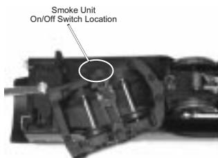
Figure 3: Smoke Unit Switch
