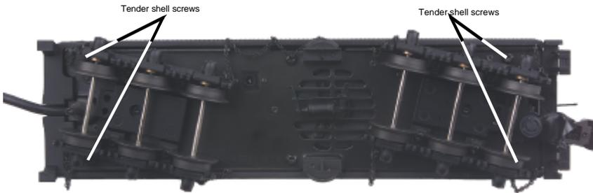
*Figure 9. Screws to remove the tender shell*
