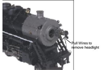
*Figure 8a. Replacing the Headlight*
