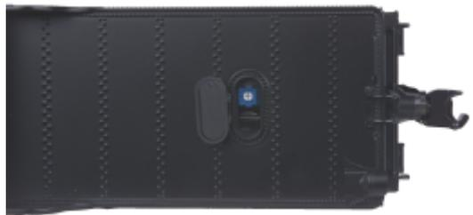
*Figure 2. Manually Adjusting the Proto-Sound 2.0 Volume*
