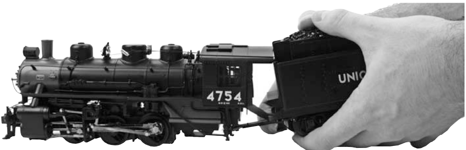
Figure 4: Connecting Locomotive to Tender
