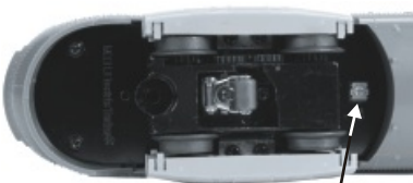
Smoke Unit Control
