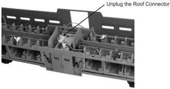
To replace the interior lights unscrew the light boards and remove and replace the entire assembly.
