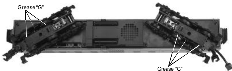
Figure 4: Greasing The Chassis Trucks
