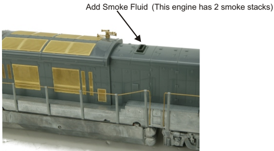
Figure 2. Adding Smoke Fluid
