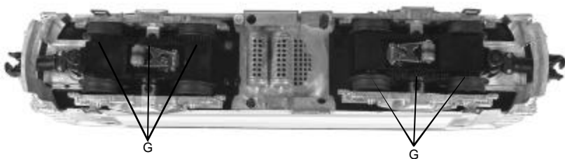
Figure 8: Greasing The Power Trucks
