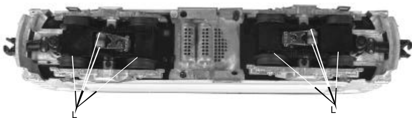
Figure 7: Lubricating The Truck
