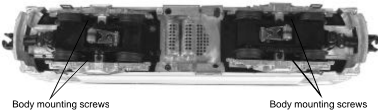
Fig. 9 Removing the body mount screws
