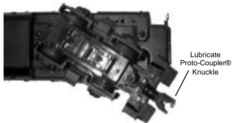
Figure 2: Lubricating The ProtoCouplers
