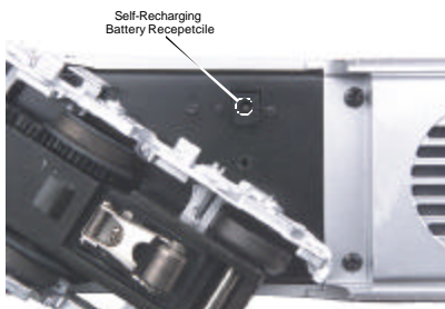
Figure 9: Battery recharging port
