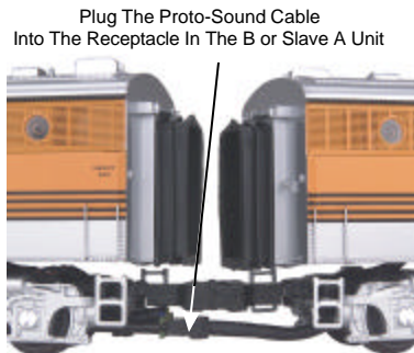
Figure 4: Connecting the engines
