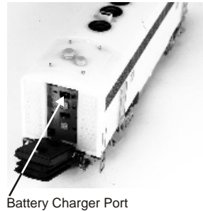
Figure 9. Battery Charger Port location.
