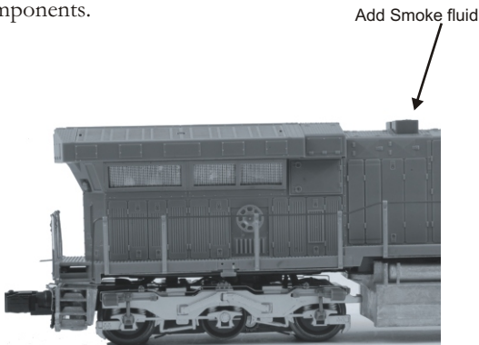
Adding Smoke Fluid
