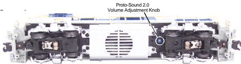
Figure 1. Proto-Sound 2.0 Volume Adjustment Knob
