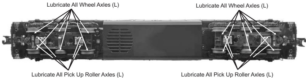
Figure 1: Lubrication Points on the Locomotive
