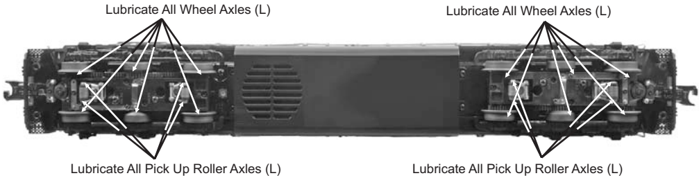
Figure 8: Lubrication Points on the Locomotive
