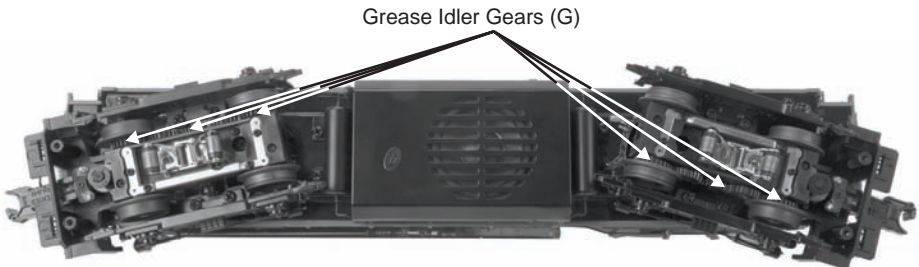
Figure 11: Greasing The Idler Gears
