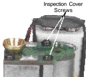
Figure 12: Smoke Unit Inspection Cover
