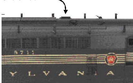
Figure 11: Adding Smoke Fluid
