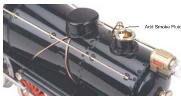
Figure 3: Adding Smoke Fluid
