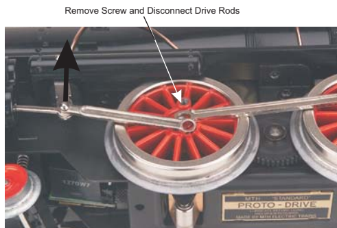
Figure 8: Disconnecting Drive Rods
