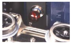
Replace the red firebox lamps with M.T.H. CI-000007 red lamps.
