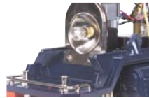
Replace the headlamps with M.T.H. CI-0000001 clear lamps.
