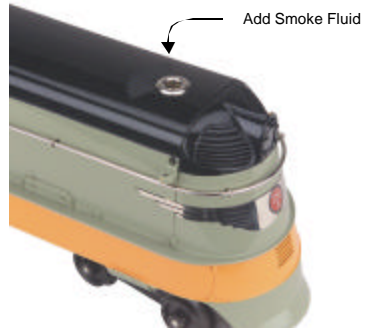
Figure 3: Adding Smoke Fluid
