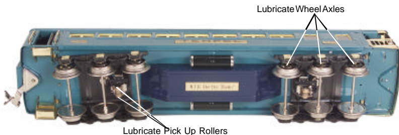
Figure 1: Lubricating The Trucks
